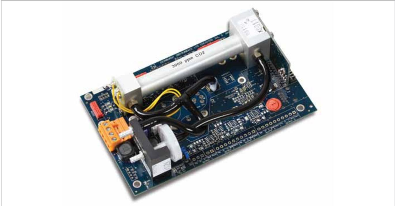
The OEM Gascard<sup>®</sup> NG infrared gas sensor, supplied by Edinburgh Sensors has been designed for easy integration into a wide range of gas detection systems where high quality, long term stability, excellent repeatability and reliable measurement of Carbon Dioxide, Carbon Monoxide and Methane gas concentrations are required.
